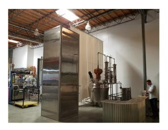
The patented Sunshiner natural distillation system is an evolutionary low temperature separation system based on the natural hydrologic cycle. In the same way that mother nature makes rain, the Sunshiner evaporates fermented mash using solar thermal energy or other low grade heat sources to create clouds of alcohol. The Sunshiner then cools the cloud creating a rain storm of high quality spirits
